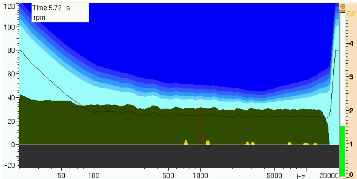
Figure 4: Sound pressure spectrum of pink noise at 45 dB(A) as in figure 1 but with loudness difference levels for the equal loudness contours from table 4.
