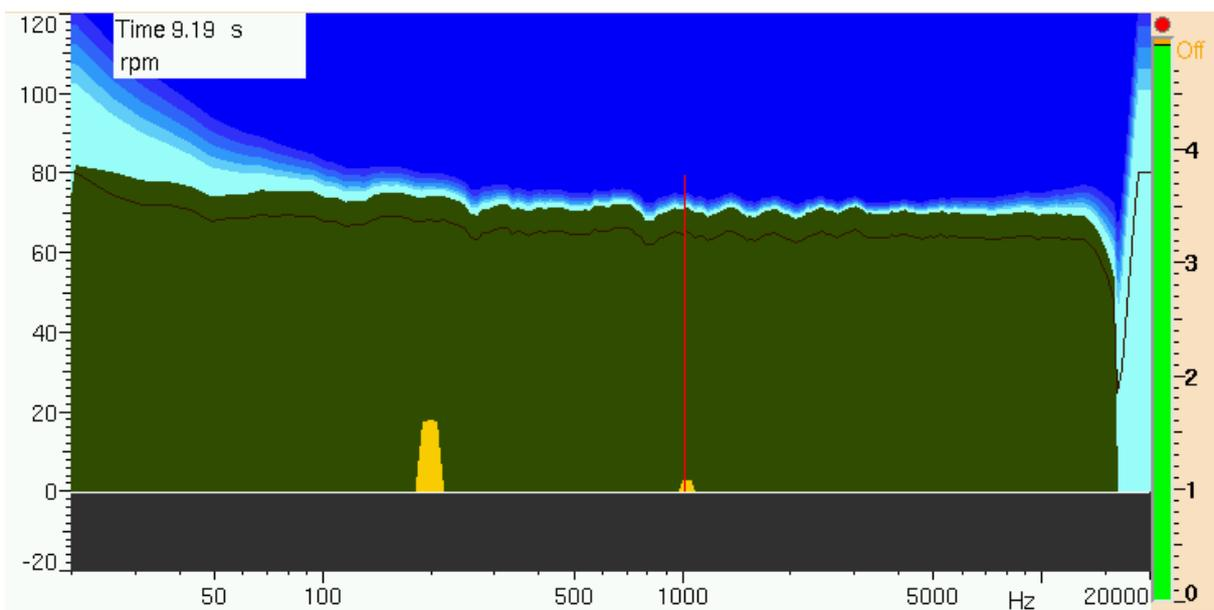
Figure 5: Sound pressure spectrum of pink noise at 85 dB(A) as in figure 2 but with loudness difference levels from table 4.
