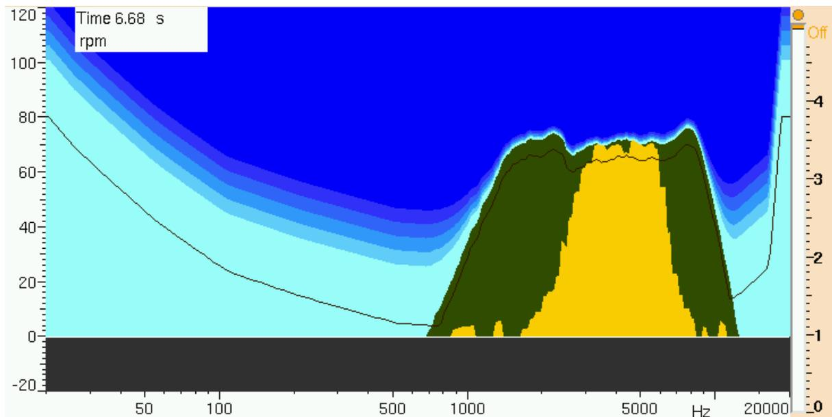
Figure 6: Noise in the range of 1500 to 8000 Hz which is 100% modulated in the range of 3000 to 6000 Hz. The noise level is shown by the green area and the modulation degree is shown by the yellow area. The height of the yellow area relative to the green shows the degree of modulation.
