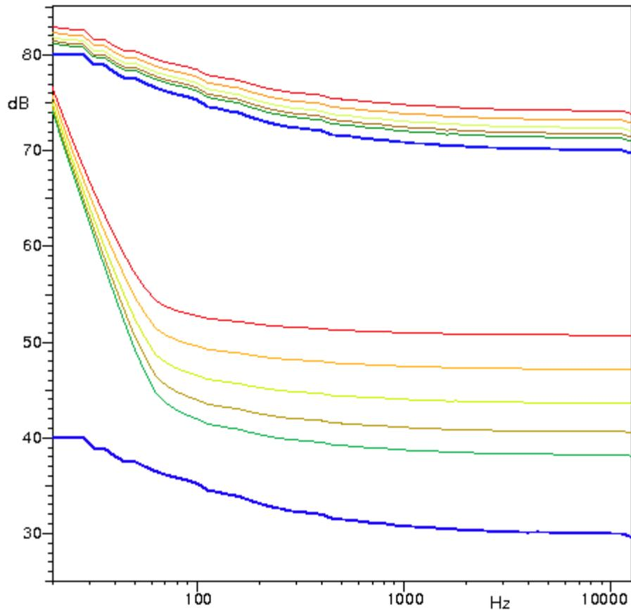
Figure 3: dB SPL levels in ERB bands for pink noise at 45 and 85 dB(A) (thick blue curves) together with the equal loudness level curves at both levels shown for the Sone differences from table 4. The curves with colors green, brown, yellow, orange and red are equivalent to the loudness of tones in quiet with the dB SPL values of 25, 30, 35, 40 and 45 dB.
