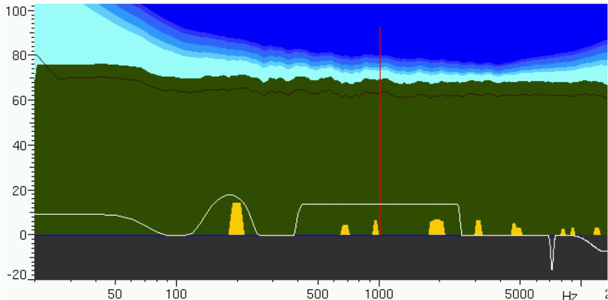
Figure 7: possible filter forms to be freely applied on noise, tones and even modulation: frequency step, smooth band filter, sharp band filter, narrow filter
